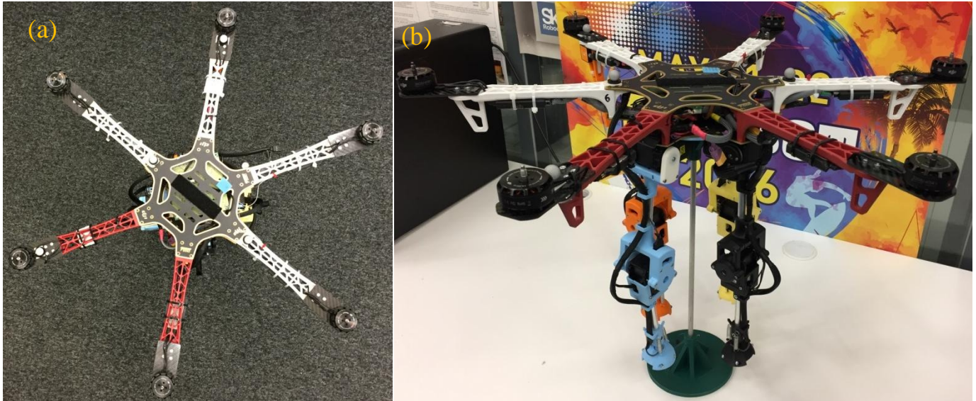
Figure 2. Quadruped mobile robot with: (a) Flying system, (b) four-legged drone whole body
