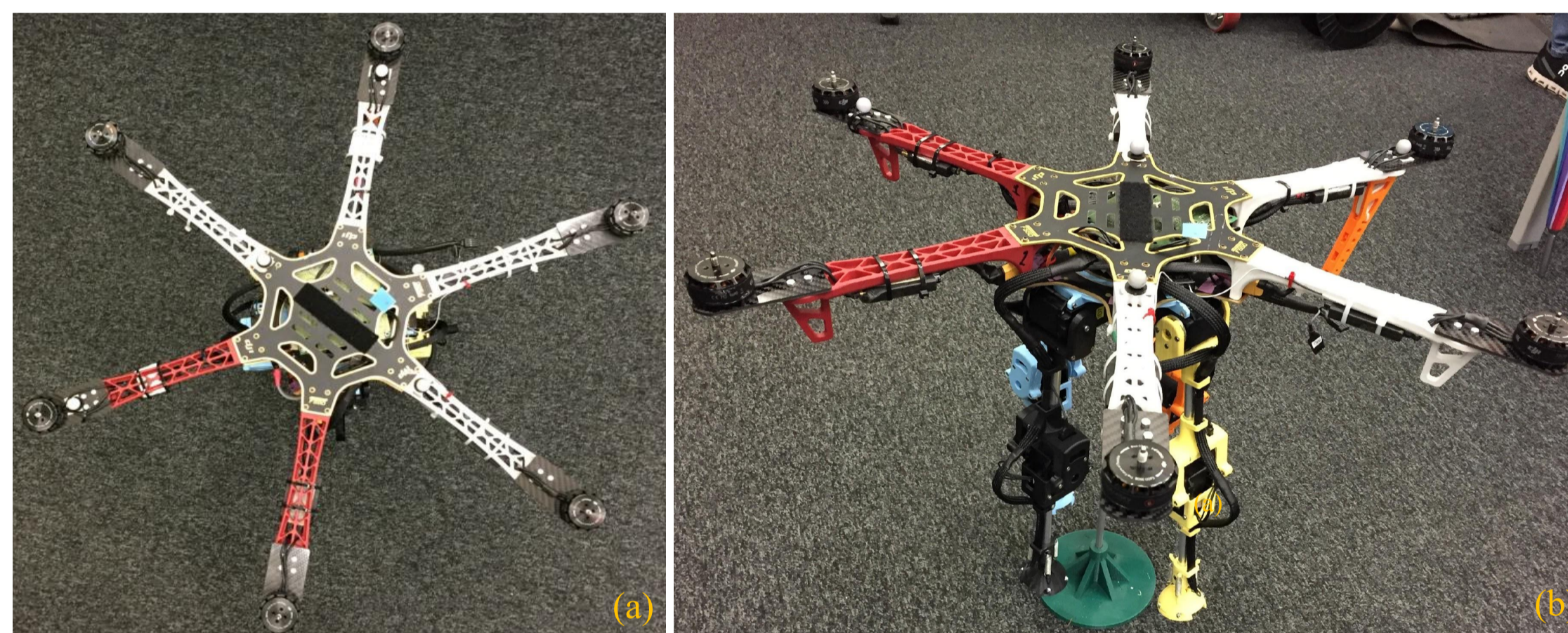
Fig.1 Quadruped mobile robot with: (a) Flying system, (b) four-legged drone whole body
